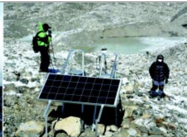
Figure 5.8: Field Server with solar panel at Imja Glacier Lake 8
